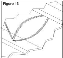
The speaker wire is looped and hung on two nail attached to the joists securing it for future use. Make sure the location is noted on house plans.
